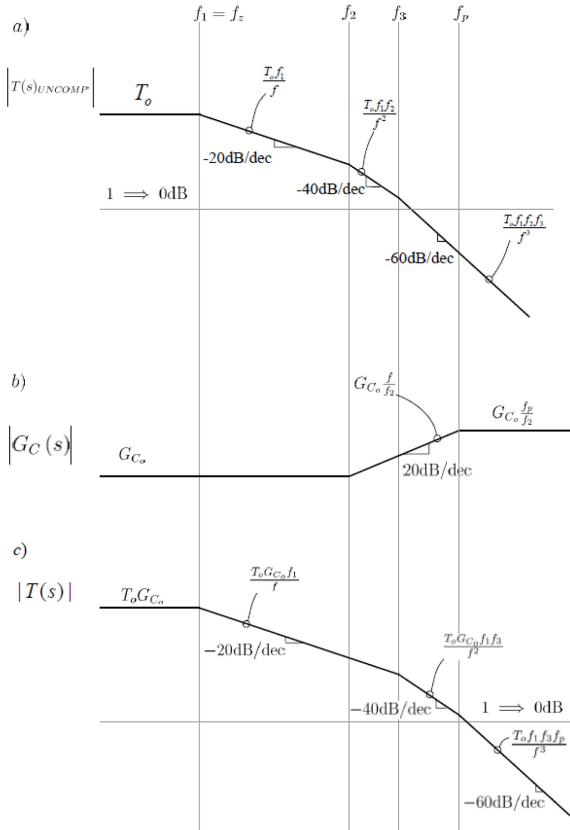
Figure 5.20: Lead Compensation Magnitude Construction
