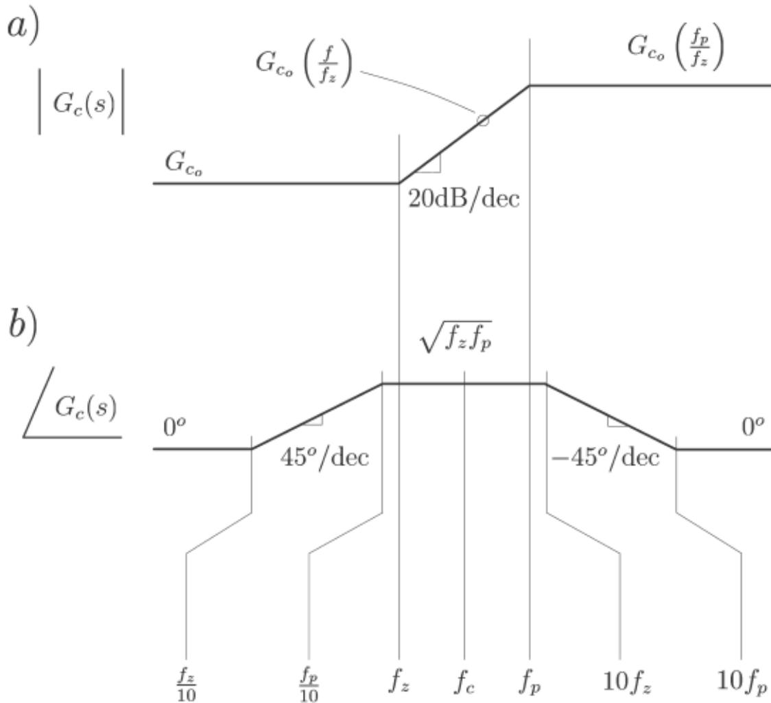
Figure 5.19: Bode Diagram: Lead Compensator
