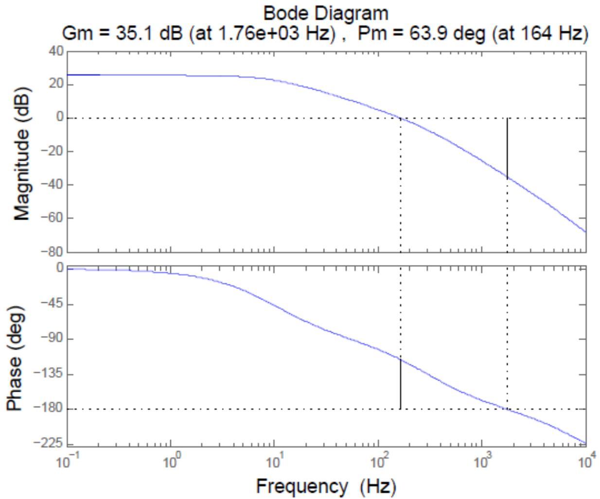
Figure 5.22: Matlab Analysis of Lead Compensated System
