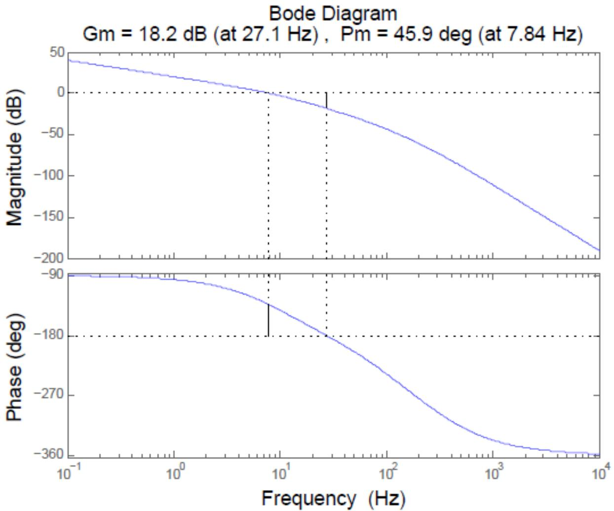
Figure 5.11: Matlab Analysis of Dominant Pole Compensated System
