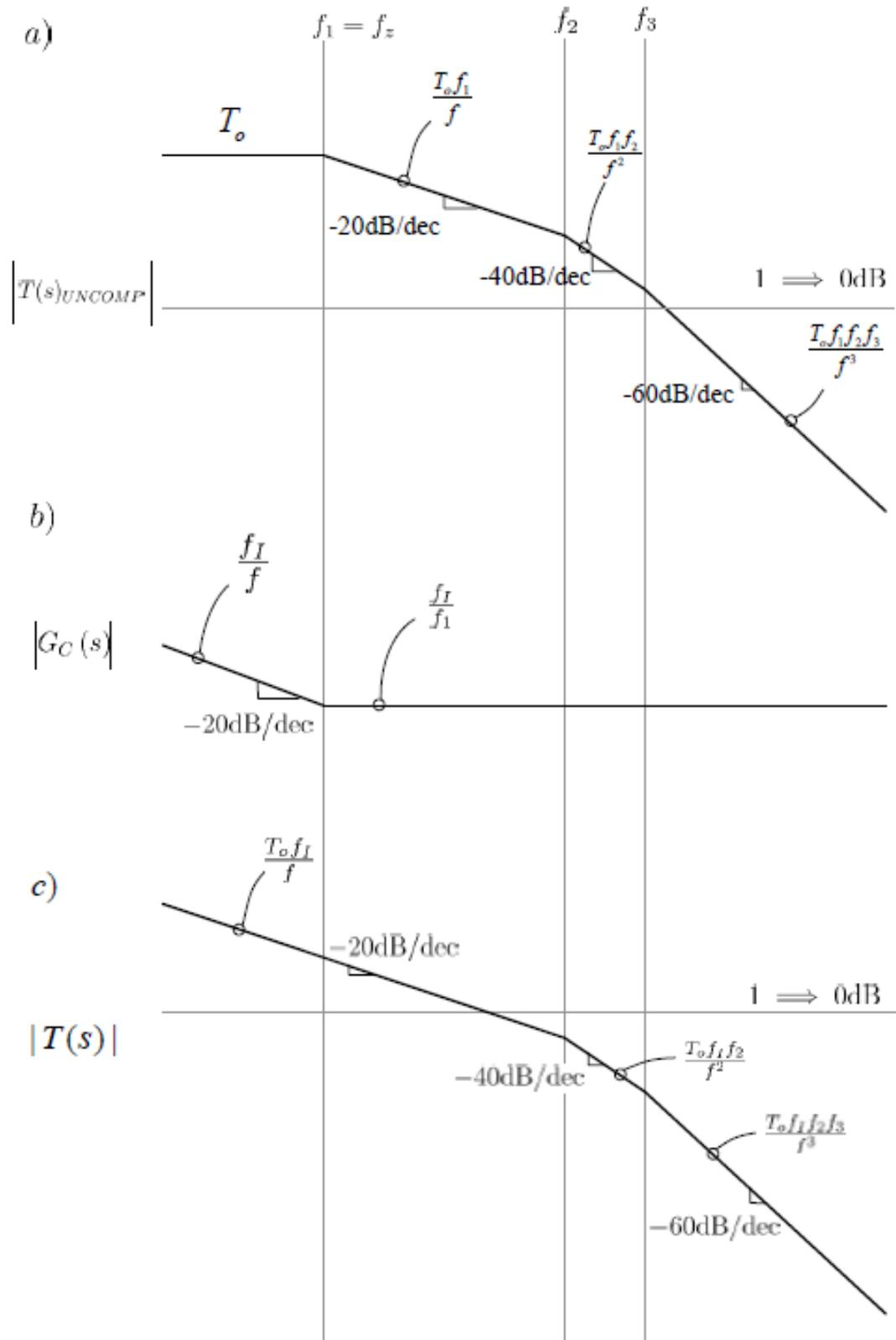
Figure 5.13: Dominant Pole with Zero Magnitude Construction
