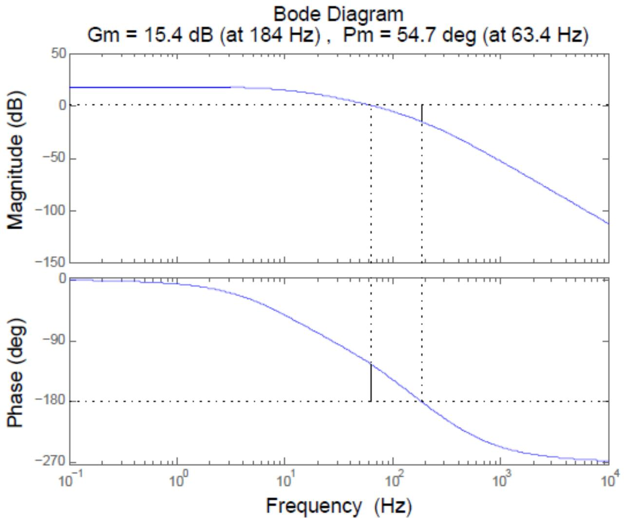
Figure 5.5: Matlab Proportional Compensated Loop Gain Bode Plot
