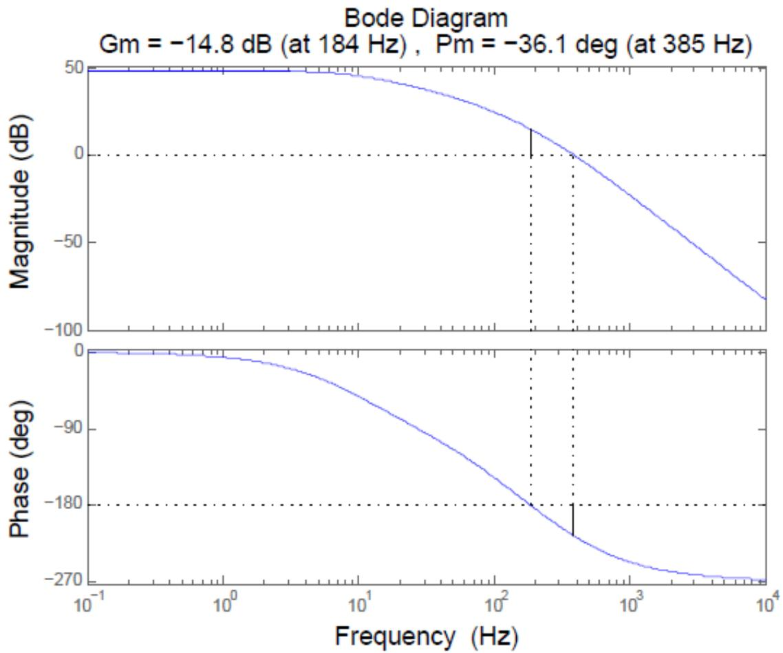
Figure 5.3: Matlab Analysis of Uncompensated System
