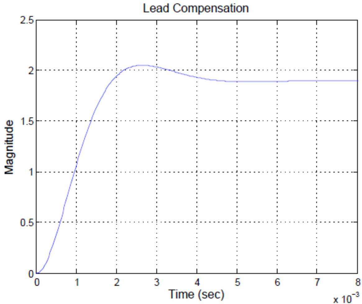
Figure 5.23: Step Response of the Lead Compensated System
