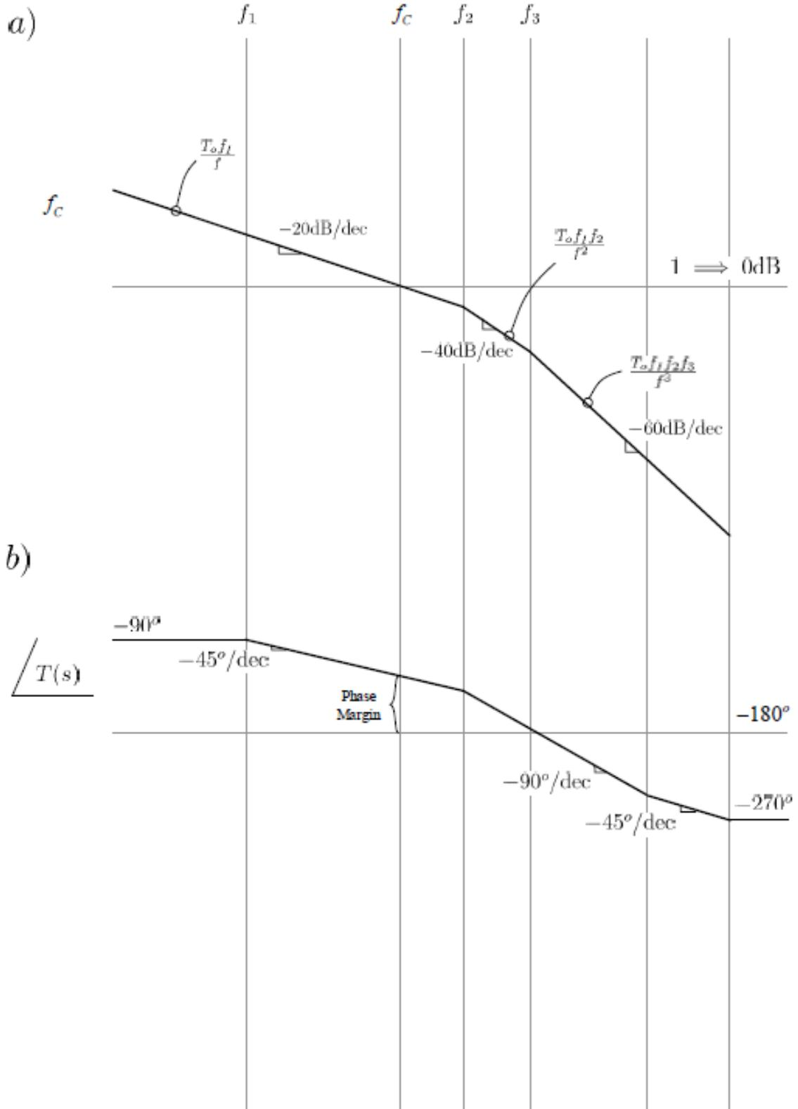
Figure 5.14: Dominant Pole with Zero Compensated System
