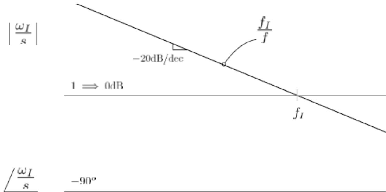
Figure 5.7: Bode Plot: Dominant Pole Compensator
