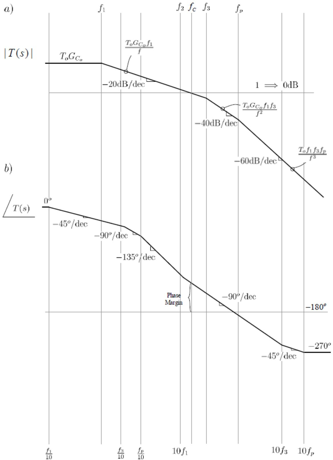
Figure 5.21: Lead Compensated System
