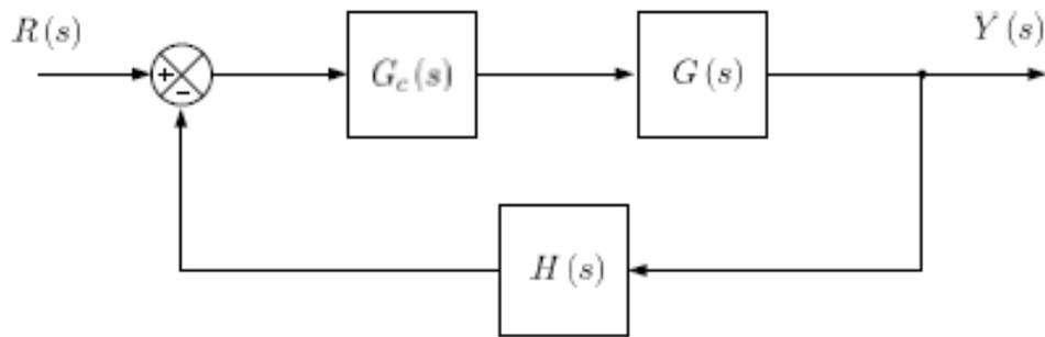
Figure 5.1: Feedback System Block Diagram
