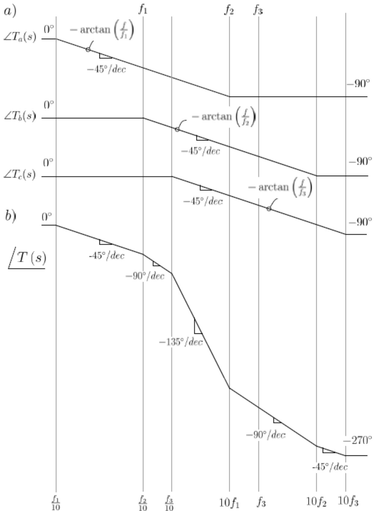
Figure 4.12: a) Asymptotic phase plots for the constituent transfer functions, b) Asymptotic plot plot for the composite transfer function
